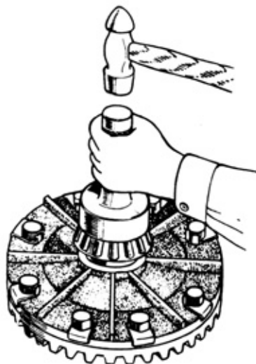
Fig. 4-36 Installing Side Bearing Cone
